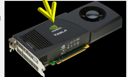
Tesla S1070 (above) containing four NVIDIA C1060 devices (right) with 240 processors per device.
