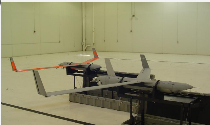
Image of the Dual Bay ScanEagle (forward) and the Single Bay ScanEagle (back).
