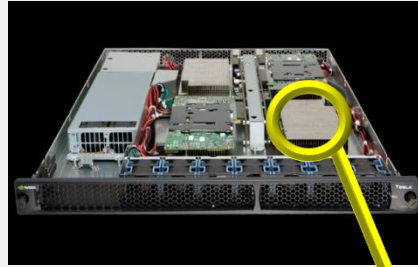
Tesla S1070 (above) containing four NVIDIA C1060 devices (right) with 240 processors per device.
