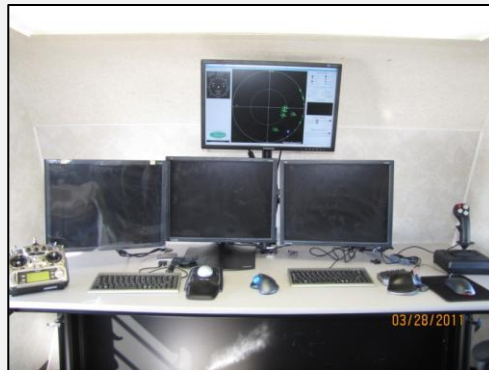
Image of the ScanEagle GCS with integration of the GOIDS (top monitor).
