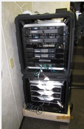
Computer system that runs the GPAR-RMS visualization and fusion systems.
